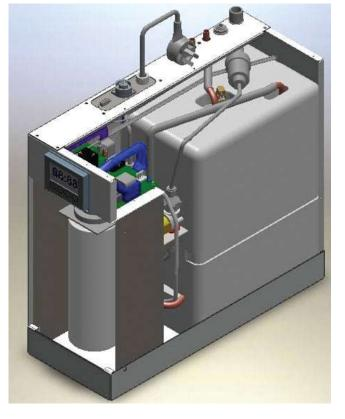
**An inbuilt filter** is factory fitted to all Rheem "TB" models both 3 and 5 litre. This 5 micron filter will require replacement every 4000 litres of use. The filter is installed to remove chlorine, taste and odours for a perfect drink of water or cup of tea. Fine dirt and sediment particles are also removed and a phosphate compound reduces costly lime-scale build up.
