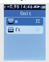
Press the **MENU** button to enter the setup menu. Use the **UP / DOWN** navigation buttons to highlight the DIST option. Press the **Enter** button.
