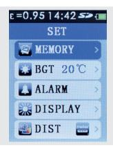
If required, the ALARM setting allows user to preset either or both a high and low threshold temperature alarm. A tone will sound when the high / low thresholds are viewed.
