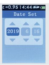
Press the **MENU** button to enter the setup menu. Use the **UP / DOWN** navigation buttons to highlight the **DATE** option. Press the **Enter** button.
