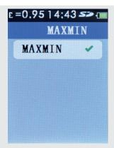
The **MAXMIN** setting, when enabled, indicates the position of the highest and lowest temperatures as well as their values at the bottom of the LCD display.
