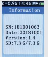
The setup option **INFO** displays the camera serial number, date of manufacture, firmware version and size of the fitted micro SD card.
