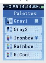
The **PLT** setting allows a user defined choice of the thermal display palette on the LCD displayed images.
