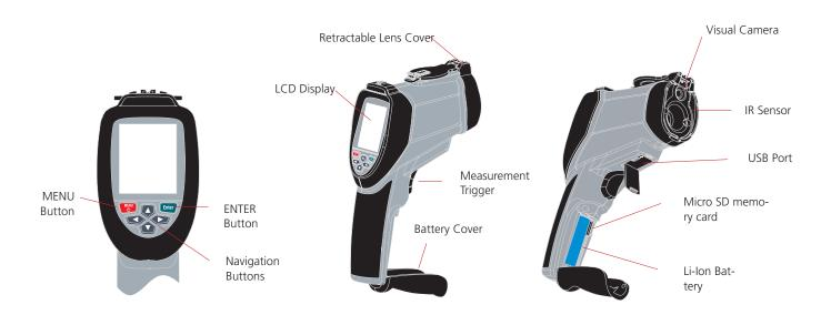
Note: Micro SD card MUST be inserted to store any images. The SD card symbol will be visible at the top left of the LCD screen next to the battery symbol.
